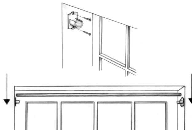
Using a pencil, mark the position on both sides of the window frame where the mounting plates will be attached. The height is determined by the window treatment being placed on the rod. Attach with the screws provided making sure the mounting plates are aligned and level with one another. Each side of the rod can now be dropped into the mounting plates.
