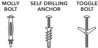
**WALLBOARD OR PLASTER:** Hollow wall applications: Use a secure fastener designed specifically for this purpose.
