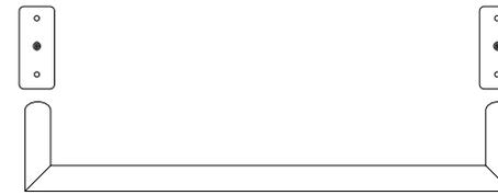
Unscrew the backplate from rod. Place panel or rings on rod and then screw on backplates to rod ends. Center the rod over the window opening. To ensure it drapes at the correct length, hold the rod up to the spot you wish to install it. Raise or lower your treatment as desired.
