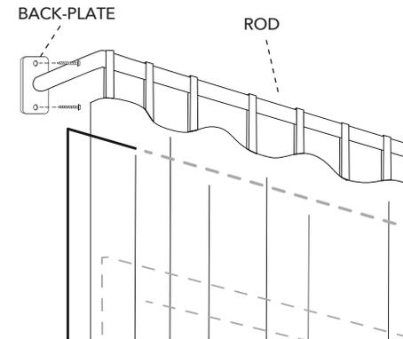
After you have located the ideal location, make sure the rod is level and use a pencil to mark the screw holes in the backplates above the window or door frame where the brackets will be mounted. If you received a center support bracket place it in the middle point between the two backplates and mark the screw holes in it as well.
