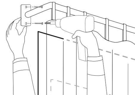
Once you have established where everything should go, pre-drill the holes in their assigned spots, making sure it is the right depth for the supplied screws. Install the return rod with the backplates attached, using the screws provided.
